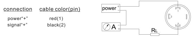
wiring drawing of 2-wire 4~20mA output (hirschmann connector)
