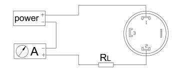
wiring drawing of two-wire 4~20mA output (hirschmann)
