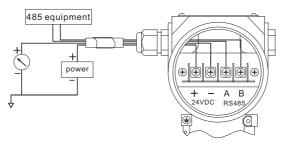
electrical connection for RS485interface (MODBUS protocol)
