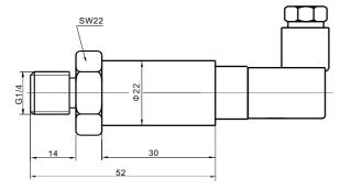
inner cavity type(diameter: 22mm)
