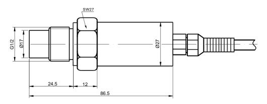
flush diaphragm type (range: 0~10... 1200bar, suitable for the measurement of fluid with grains such as slurry etc)
