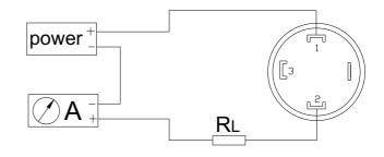
wiring drawing of two-wire 4~20mA output (hirschmann)
