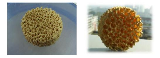
AGS-Industrial Zirconia Ceramic Foam Filters (CFF-ZR) is available in all common sizes in the range of 40x40x20mm up to 150x150x30mm. Round filters are available from D40x20mm up to D150x30mm. Although PPI 10 is the porosity most commonly used for steel casting, finer porosities up to PPI 60 are available on request. Custom-made cut-to-size filters are also possible.
